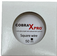
R930019C Square wire 50 m, 0.6 mm spec. for cut-out systems Tensile strength 170 kg/1700 N. Very flexible.
